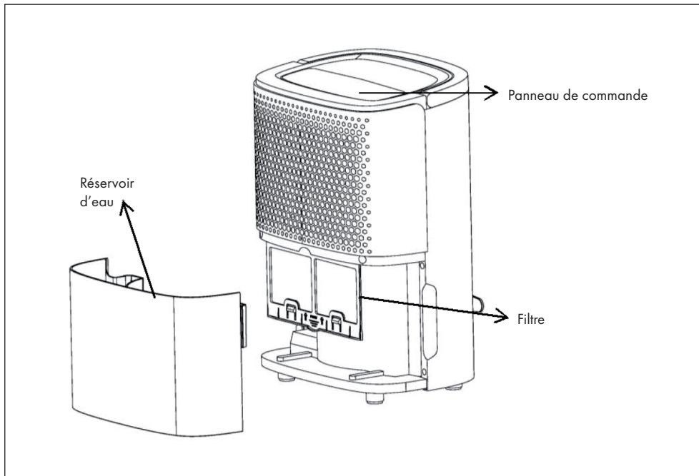
**Dos de l'appareil**
